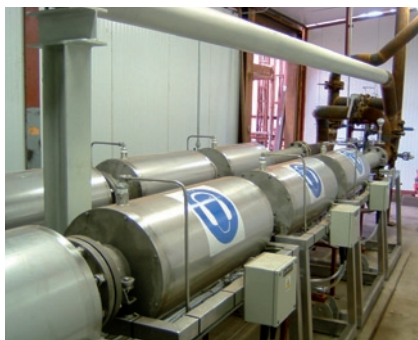
Prosonitron™ sonocrystallization technology at large scale in continuous flow (Courtesy of Prosonix Ltd, Oxford UK)
