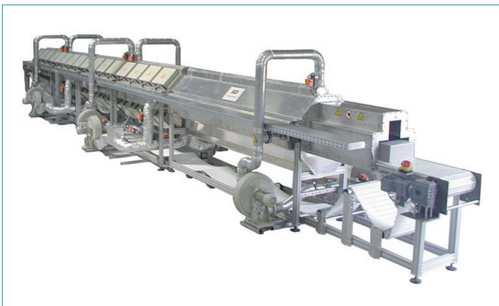
Microwave hybrid continuous belt dryer
