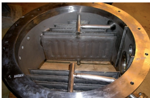
Heat transfer panels in a pilot HIDiC column (Courtesy of Delft University of Technology)
