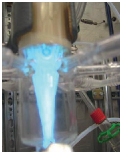
Stripped optical fibres used in photocatalytic reactor (Courtesy of Delft University of Technology)
