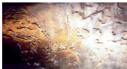
Liquid flow on spinning disc surface (Courtesy of University of Newcastle)
