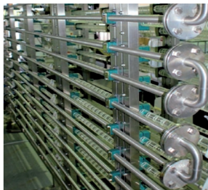
Oscillatory Baffled Reactor (Courtesy of Ni-Tech Solutions Ltd.)
