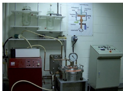
Spinning Disc Reactor setup (Courtesy of Clarkson University)
