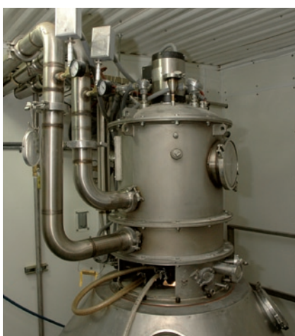
Rotary-valve pulse combustor mounted at the top of the spray dryer
