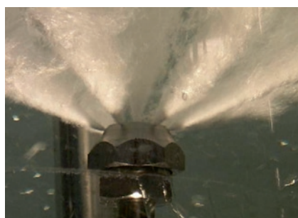
Transonic oxygen injection in fermentation plant (Courtesy of DSM)
