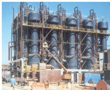
Pulsed columns for metal extraction (Courtesy of Bateman Litwin N.V.)
