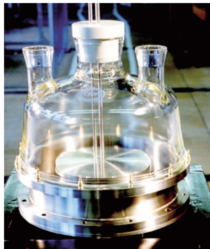
Spinning Disc Reactor setup (Courtesy of University of Newcastle)
