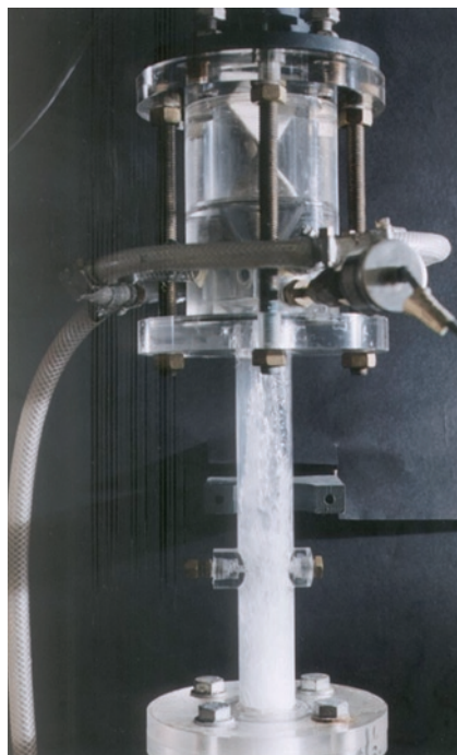
Ejector reactor (Courtesy of BHR Group Ltd.)
