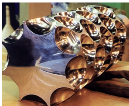
Cavity transfer mixer rotor (Courtesy of Maelstrom Advanced Process Technologies Ltd.)
