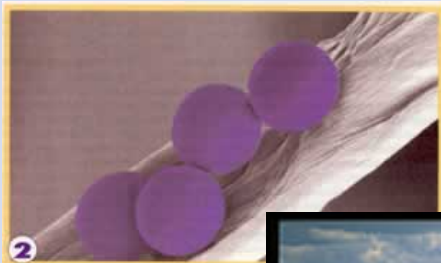
Figure 2: A 5 micron bead on a HEPA filter fiber
